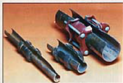
Typical compression couplings and steel pipe split by Bullet.
